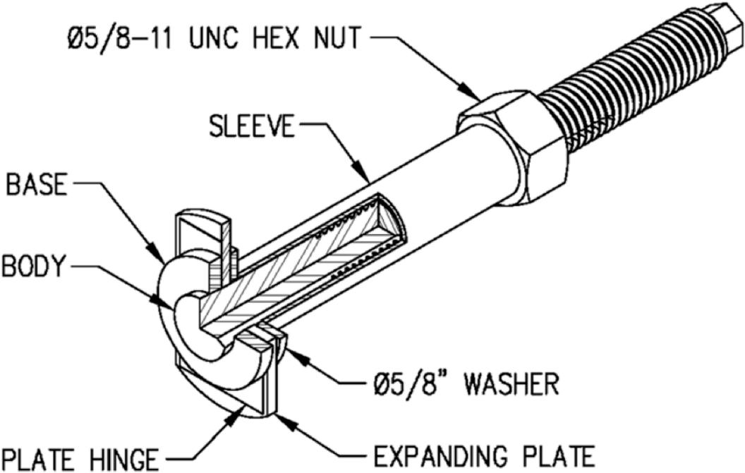
Figure 1: Hybrid Anchoring System
