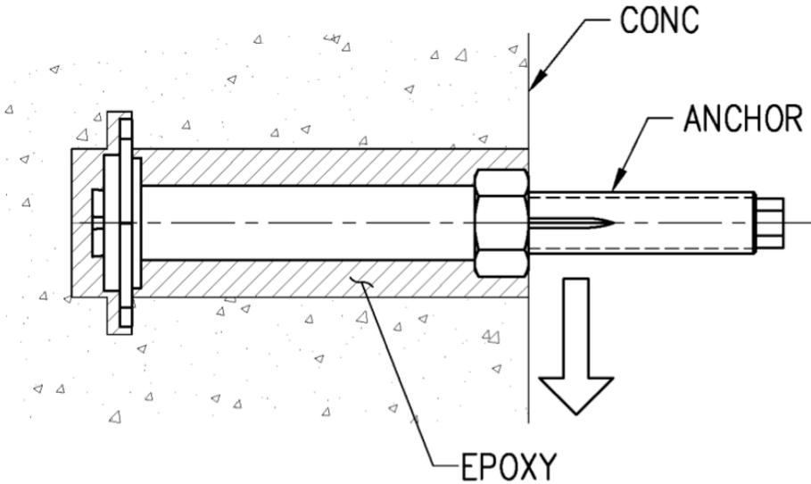
Figure 6: Shear Test, With Adhesive
