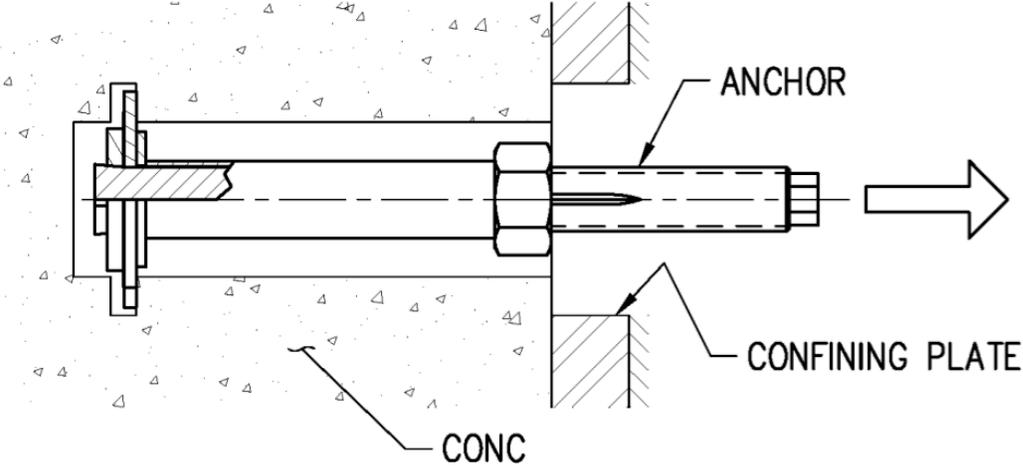
Figure 4: Tension Test, No Adhesive
