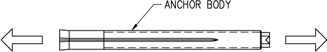
**Figure 8: Body Tensile Strength**
