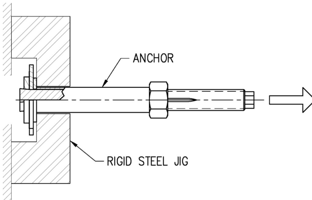
**Figure 3: Pullout Strength Test**
