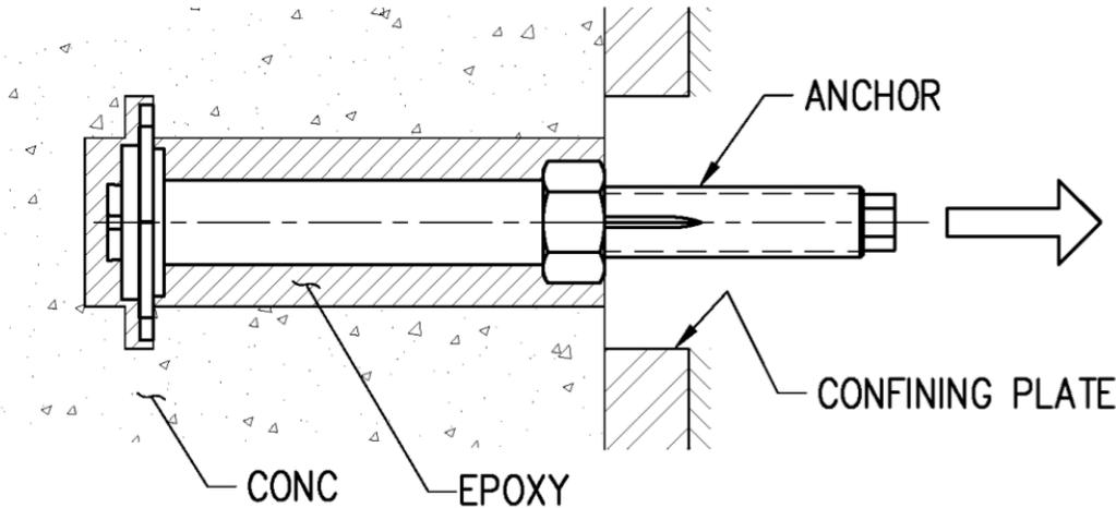
Figure 7: Confined Tension Test, With Adhesive.
