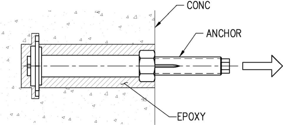
Figure 5: Unconfined Tension Test, With Adhesive
